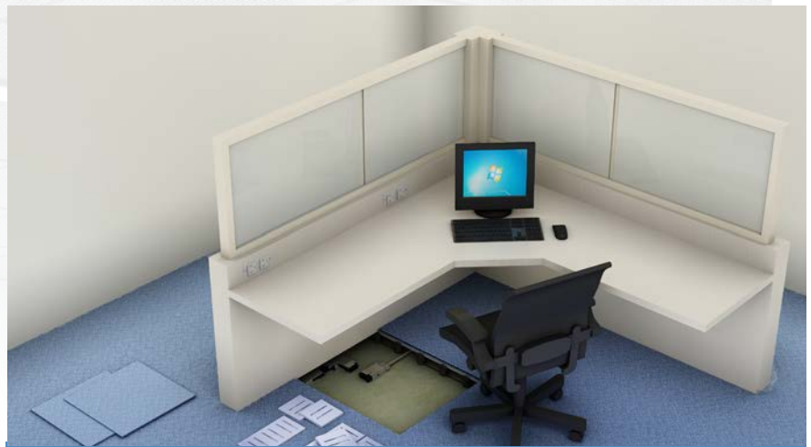
Power to Systems Furniture
