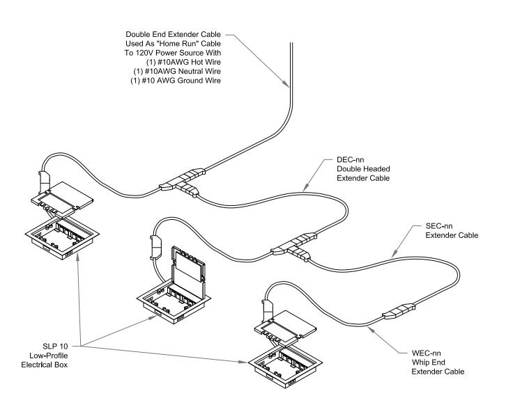
The DEC-nn Double End Extender Cable Has (1) 20A/120V Circuit Available. The Above Illustration Shows A "Daisy Chain" Application On One 20A Circuit Only
